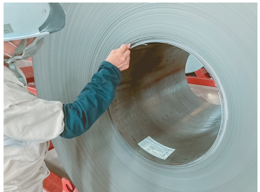
Off-gauge area is identified by mark drawn on the edge.
