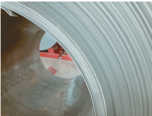
Approx 13m of "not-rolled-to order" sheet (off gauge) is in inner side of the CRFH.
